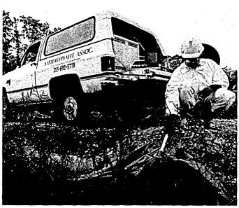
Satterthwaite uses state-of-the-art mobile equipment mounted in the back of a four-wheel drive vehicle to perform necessary testing on-site. Instead of weeks, we can deliver results for organic contamination immediately. And regulatory agencies recognize our methods as excellent for field screening purposes. situations that can limit liability and supply early warning against the potential for financial hazards.
